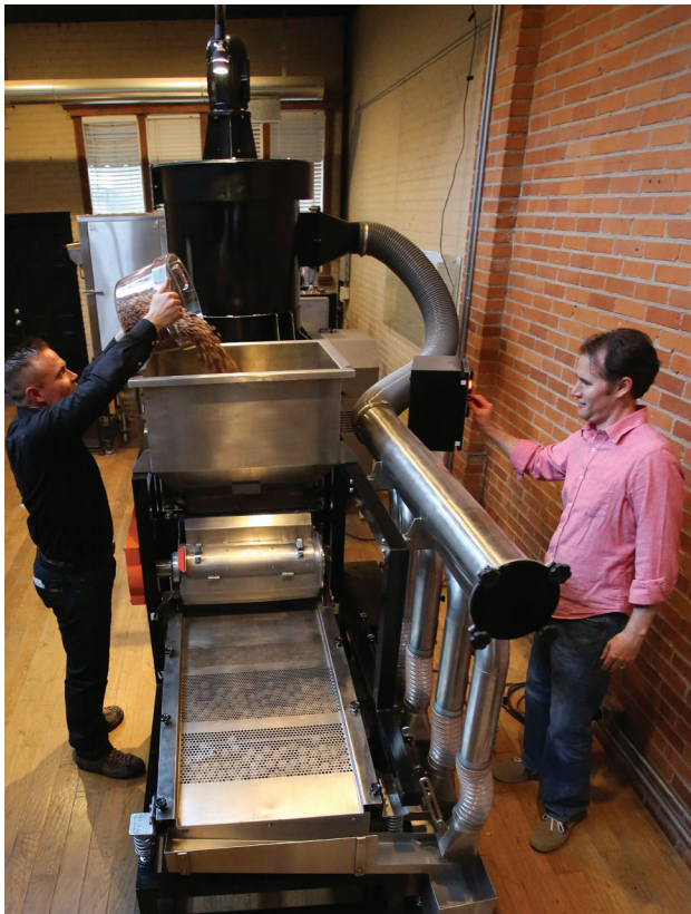
Coleman and Davis beansmiths Phil Davis (left) and Morgan Coleman proudly pour beans into their new JAF Inox winnower.
