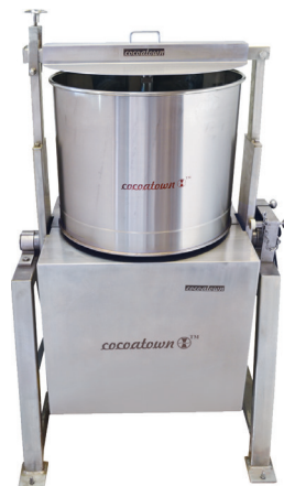
ECGC-65A Grindeur Specifications: Capacity 65 lbs. of nibs to yield up to 100 lbs. of chocolate liquor, depending on recipe; multi-purpose, can grind almonds, hazelnuts, pistachios, etc. to make nut butters.
