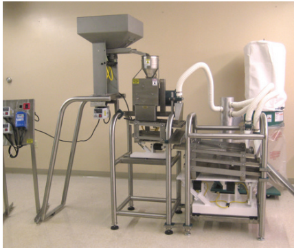
Cacao Cucina Winnower (WINN-45) Specifications: Capacity: 45 kg /100 lbs of roasted beans per hour; pressure adjustable, variable speed bean breaker; three vibratory product screens; separate fines delivery; vacuum system for shell debris. Stainless steel breaker, product screens, discharge chute and frame.
